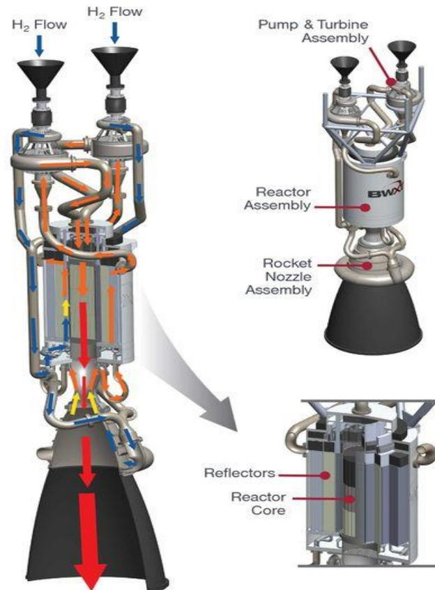
A nuclear thermal propulsion engine diagram with arrows that show the flow path of the hydrogen propellant. The arrow colors represent the relative gas temperature, with blue as the coldest and red as the hottest.
